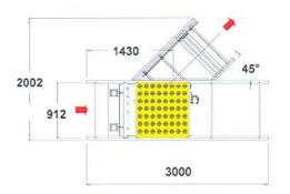
The Switch Sorter is independently driven from a 0.37kW. SEW Motor, to give either 60 m.p.m. or 110 m.p.m. maximum linespeed of Sorter Wheels. We recommend that an Inverter is fitted to the gearbox to enable fine tuning of module.
